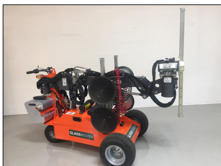
Figur 9 GLASSMOVER i transportstilling.
