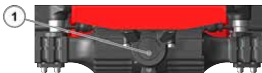
Figur 149: Kontrollér forakslens differentiale for lækager
