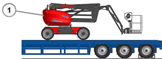
Figur 122: Maskine i transportposition (1) - 160 ATJE S1 - 160 ATJE RC S1
