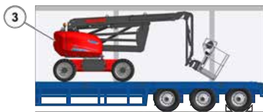
Figur 135: Maskine i sammenfoldet position (3) - 180 ATJE S1 - 180 ATJE RC S1
