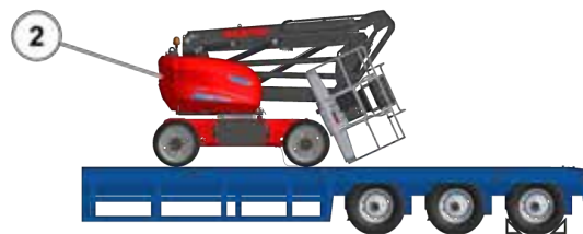
Figur 124: Maskine i sammenfoldet position (2) - 160 ATJE S1 - 160 ATJE RC S1
